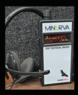
Hawk Radio is a compact DIS (Distributed Interactive Simulation) based device that enables representative communication in a simulation environment generating "train as you fight" scenarios.
