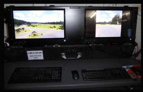
SIMSTATION is a Portable Role Training System, developed by MINERVA in partnership with D3A Defence. This mobile self-contained simulation station enables end to end synthetic training in a Live Virtual and Constructive (LVC) environment. PRTS is available in several configurations including single and dual screen and with up to 3 embedded PCs.
